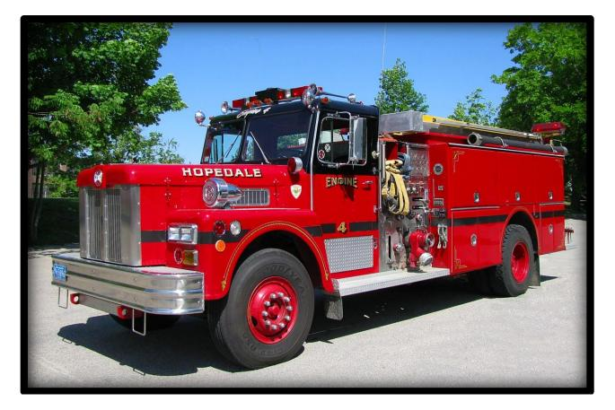
1987 "S" Model Maxim, 2-man cab, 1,000 gallon water tank, 1,000gpm pump, 30 gallon foam cell, 23,835 miles, VIN # 35-3007. Refurbished body in 2002. Original Engine and Pump. Has a cracked transfer case and needs steering box rebuilt. The Town does not provide any guarantees or warrantees, therefore, the truck will be offered on an "as is- where is" basis.
